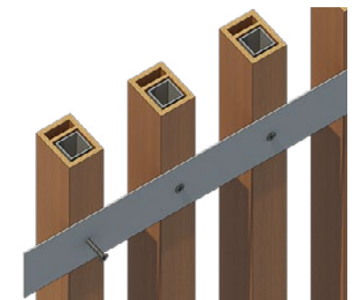
Rear fixed typical batten screen detail
